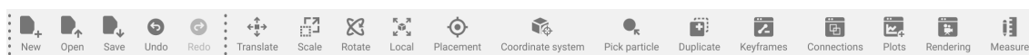
Figure 4: PreonLab toolbar. The toolbar is context sensitive and shows different options depending on the selected objects.
