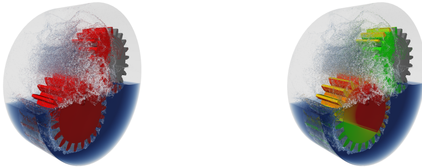
Figure 65: A gear setup after a simulation time of 0.2s. The gears start rotating after 0.1s. The wetting sensor in the left picture visualizes accumulated wetting whereas the wetting sensor in the right picture visualizes the wetting time. For the latter, the color legend is as follows: Green: > 0.0s, Yellow: 0.1s, Red: ≥ 0.2s.
